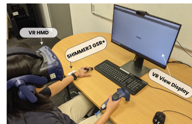
Figure 1: Experiment setup with participant wearing HTC Vive Pro Eye VR HMD and Shimmer3 GSR+ physiological sensor taking the AMT test in VR
